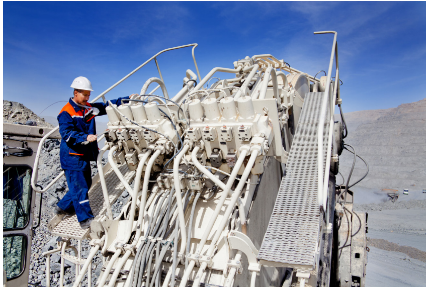
Figure 4. The complexity of hydraulic systems leads to not only difficult, error-prone installations but the likelihood of increased maintenance and associated costs.
